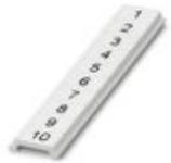
Zack Marker strip, flat, Strip, white, labeled, Printed vertically: consecutive numbers 1 ... 10, 11 ... 20, etc. up to 91 ... 100, mounting type: snap into flat marker groove, for terminal block width: 3.5 mm, lettering field size: 5.15 x 3.5 mm, Number of individual labels: 10
