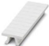
Zack marker strip, Strip, white, unlabeled, can be labeled with: PLOTMARK, CMS-P1-PLOTTER, mounting type: snap in, for terminal block width: 3.5 mm, lettering field size: 3.5 x 10.5 mm, Number of individual labels: 10
