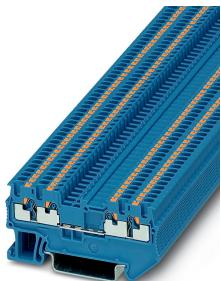
Feed-through terminal block, nom. voltage: 500 V, nominal current: 17.5 A, connection method: Push-in connection, 1 level, Rated cross section: 1.5 mm<sup>2</sup>, cross section: 0.14 mm<sup>2</sup> - 1.5 mm<sup>2</sup>, mounting type: NS 35/7,5, NS 35/15, color: blue
